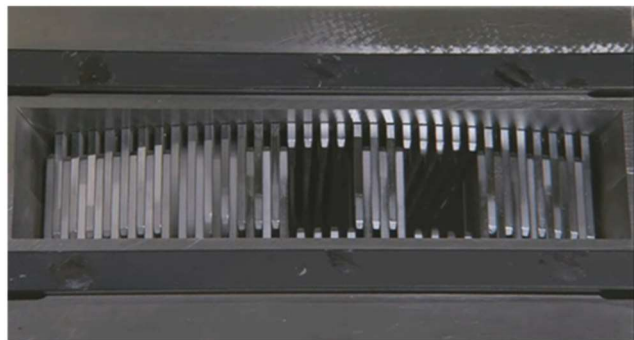
Fig. 1-2 Two Types of multi-leaf collimator [(a) standard type for conventional Linac and (b) binary type for tomotherapy]. Standard type operates by motor drive. Binary type operates by compressed air.
